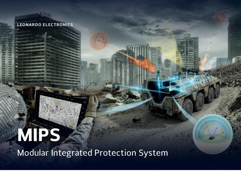
The Modular Integrated Protection System (MIPS) is being developed by a UK MoD-funded Implementation project to address active protection of military vehicles against multiple evolving threats, including Rocket Propelled Grenades (RPGs), Anti-Tank Guided Weapons (ATGWs), small Uncrewed Aerial Systems (UAS) and Electromagnetic Activities (EMA).
