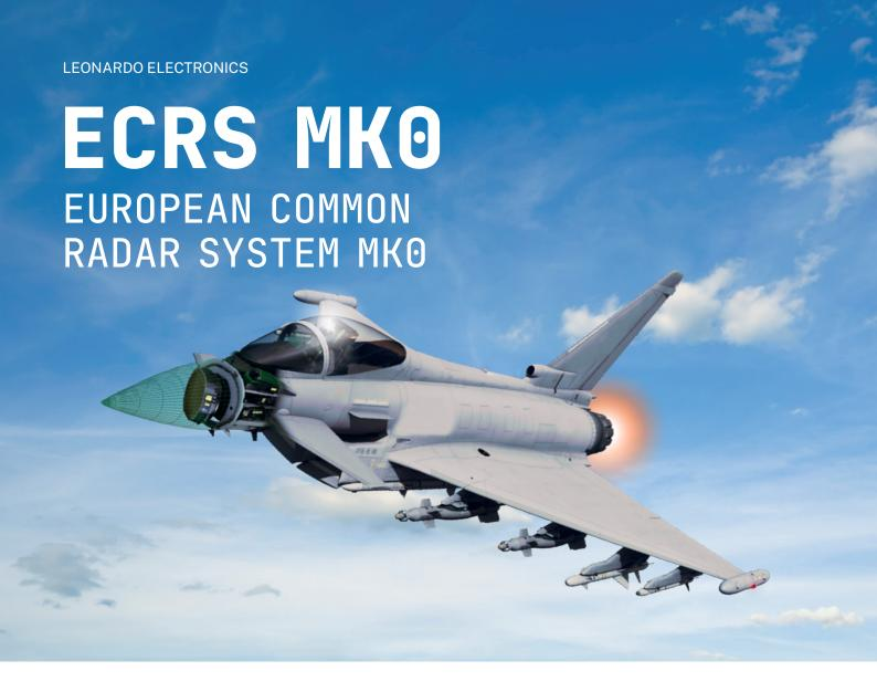
ECRS Mk0 is designed and built by Leonardo UK as part of the EuroRadar consortium, incorporating knowledge and experience gained through the development of CAPTOR-M and technical demonstrator programmes. The system, which is already flying operationally within Qatar and Kuwait Air Forces, is Eurofighter (EF) Typhoon's first AESA Radar.
